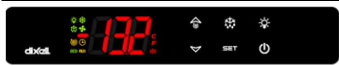
**SET**: To display target set point; in programming mode it selects a parameter or confirm an operation.
