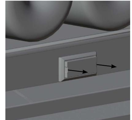
The contact switch in the housing can be levered out with a small screwdriver; it is not screwed on, but only plugged in.
