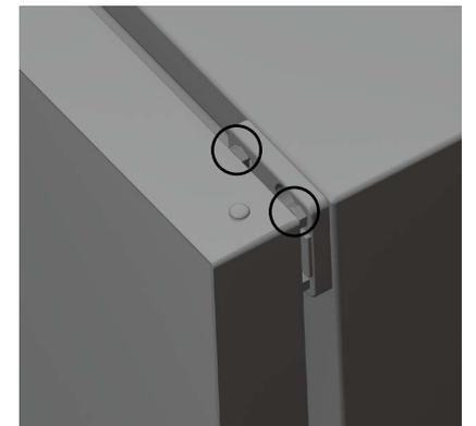
2. Then slightly loosen the hinges using a size 8 open-end wrench, align the door properly and retighten the screws.
